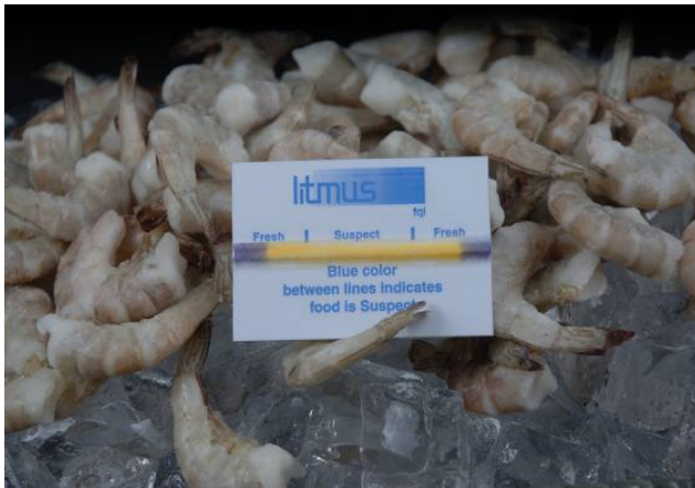
LITMUS FQI SHIPPING SENSOR SHOWING HIGH QUALITY SHRIMP WITH SOME DECOMPOSITION.
