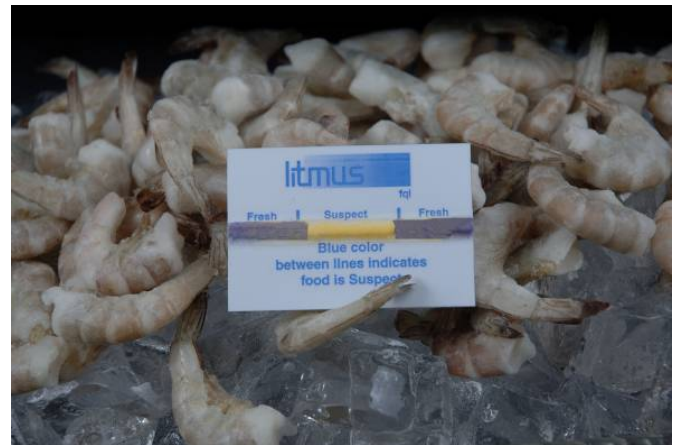
LITMUS FQI SHIPPING SENSOR SHOWING "Suspect" SHRIMP.
