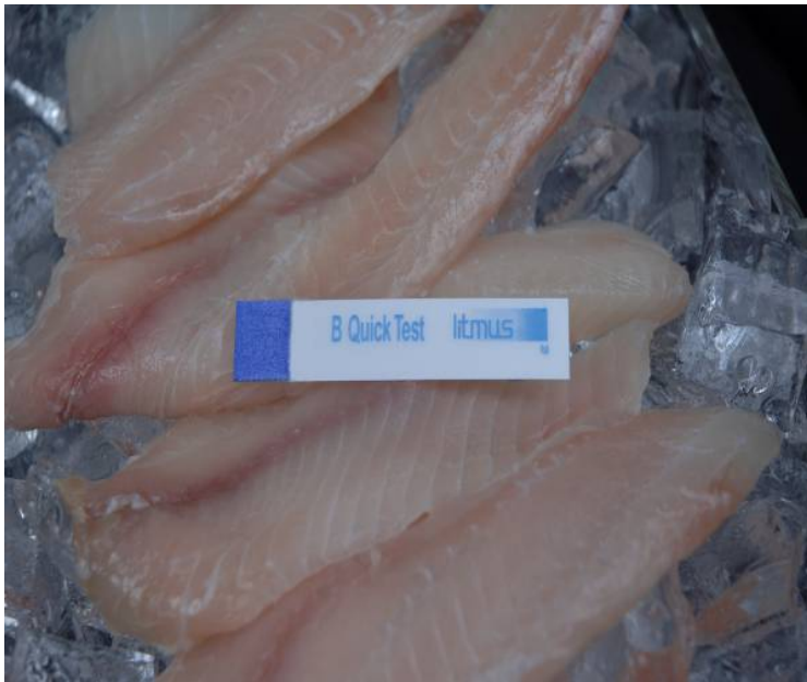
LITMUS QUICK STICK SENSOR SHOWING TILAPIA THAT IS "Suspect".
