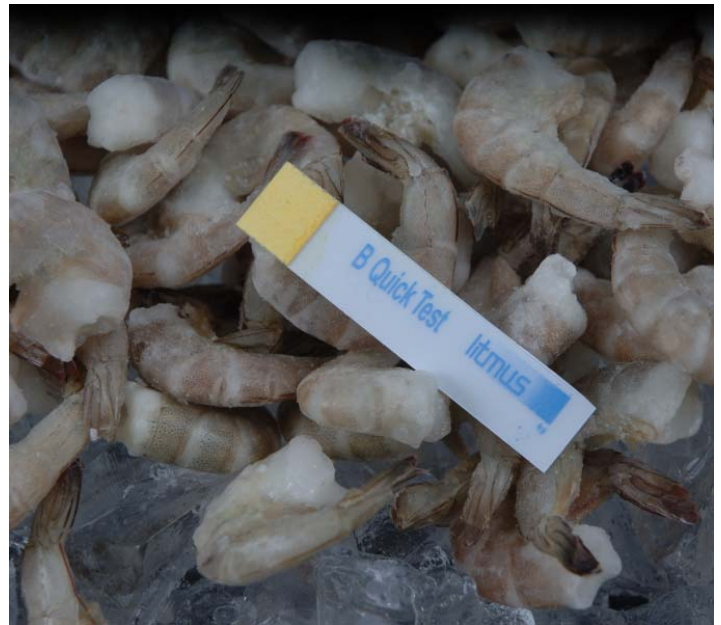
LITMUS QUICK STICK SENSOR SHOWING QUALITY SHRIMP
